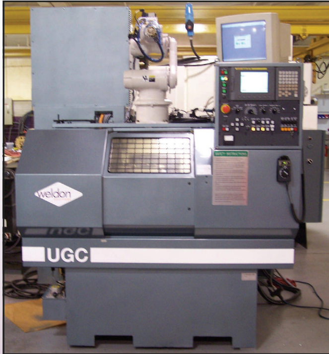
Multi-purpose chucking grinder for OD, face and ID grinding in a single set-up.
