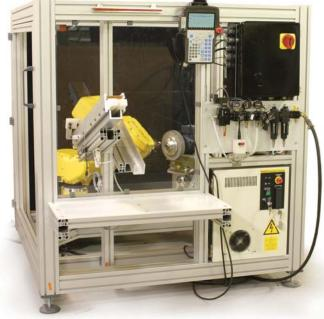
intervals in the production cycle, and a cycle speed as short as 10 seconds even when deburring multi-featured parts. The cell is surrounded by an electrically interlocked safety enclosure.
