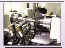
A wide variety of pins and planetary shafts ground in a single-pass process.
