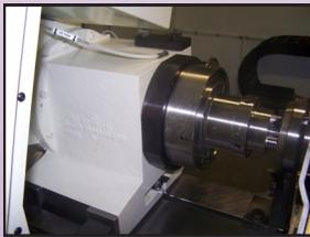
Live spindle work-head with hydraulic face driver
