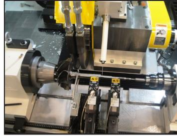
A **Renishaw** probe, presented via a pneumatic cylinder, is utilized for precise automatic lateral positioning. A table mounted in-process sizing gage from **CGI** monitors diameter size & controls the grinder in-feed until final size is achieved.
