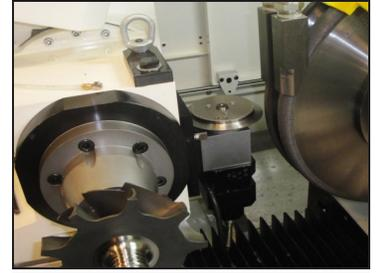
The vitrified CBN grinding wheel is dressed with a **GII** cross axis electric rotary diamond dresser aided by a **Dittel** acoustic emissions sensor to minimize wheel reduction. A custom wrap-around coolant nozzle design effectively presents coolant to the grind zone.
