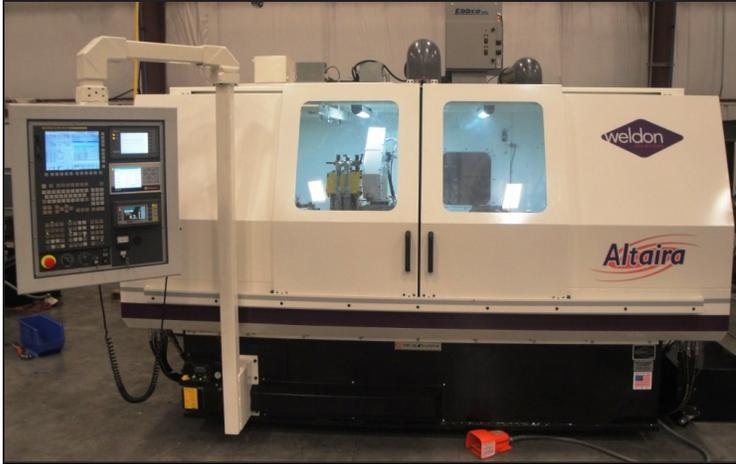
Research & Development are still a priority for a major US heavy equipment builder. The Weldon **Altaira** was selected for a test lab application to fully develop both conventional & superabrasive grinding processes. The primary reason for selection was Weldon's experience with, and the Altaira's capability for, high-speed **Peel Grinding**.
