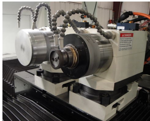
Two GMN 150mm 24,000 RPM spindles with diamond grinding wheels
