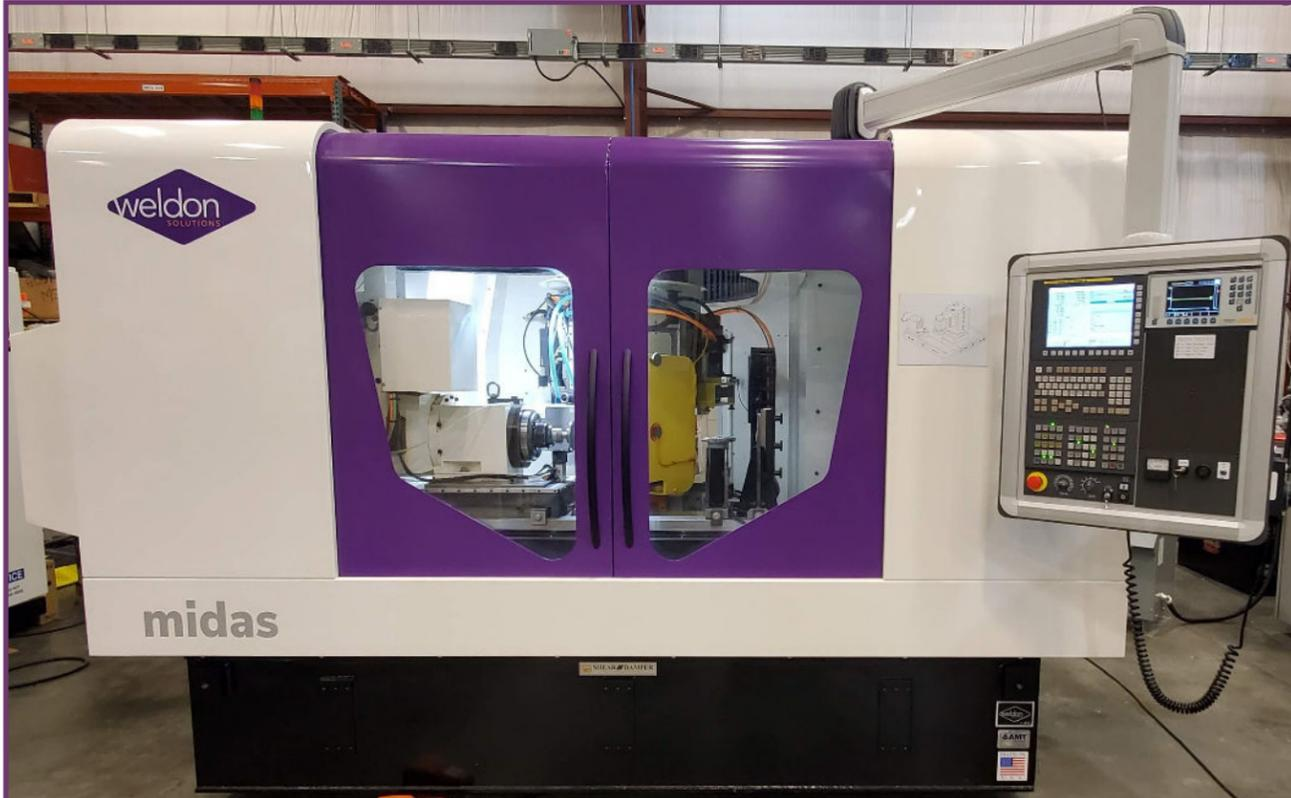
A leader in Silicon Carbide (SiC) Wafer technology has once again come to Weldon for solutions to their unique SiC boule (ingot) grinding requirements. In this application, Weldon's multi-spindle, turret based wheelhead design on the Midas platform allows for OD, Face, Flat, Notching, and Angled-Plane End Face grinding all in the same cycle.
