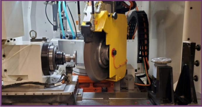
In the 1st operation, the main spindle angular approach grinding wheel is used to grind the OD and then the flat end face (dome).
