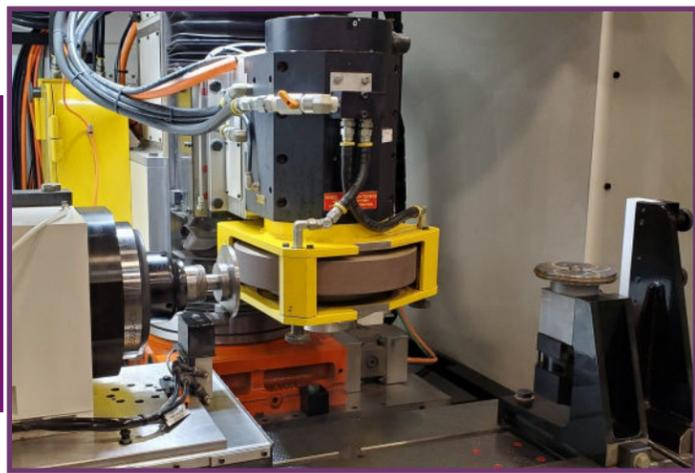
In place of a primary flat, for the 3rd operation, a notch can be ground with the fixed, vertical sub-spindle using a pre-formed wheel.
