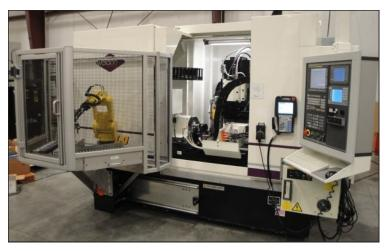
**Top Tier Automotive Steering Component Manufacturer.....**selects Weldon to satisfy demand for grinding steering gear components. Weldon's 3 in 1 process for power steering input shaft grinding allows the end user to grind longitudinal slots to a precise width, grind the major OD to size under gage control, and C-axis grind the metering edges in one continuous cycle. This results in consistent quality with an OD size tolerance of +/- .0025mm and a total cycle time under 75 seconds.
