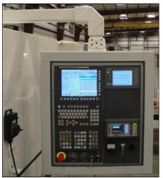
New design operator control panel featuring FANUC 32iTB CNC.
