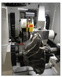
Machine arranged to accommodate impellers up to 25.5" in diameter.
