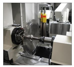
Dual plated CBN wheel pack allowed for contouring and OD recess grinding in the same set-up.
