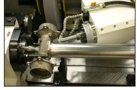
spindle with a CBN grinding wheel is presented automatically in a swing-down fixture to finish and match the body diameter.
