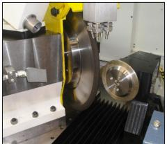
A major heavy equipment builder, and long-time Weldon customer, selected the **Altaira** for peel grinding a wide range of hardened steel pins and shafts. An angular wheelhead design was chosen to best address the more demanding shoulder grinding requirements. This is the 5th Weldon peel grinder for this customer.
