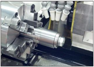
The primary spindle performs OD arbor grinding operations with part held in a manually operated 6-jaw chuck.
