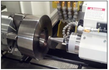
The secondary high-frequency spindle is hydraulically swung into position for diamond wheel ID die contour grinding operations.
