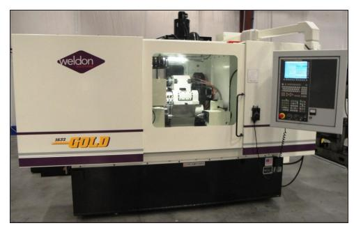
Oklahoma based manufacturer of tubing for the oil well industry receives their first Weldon CNC grinder for grinding of their dies and arbors. The machine is arranged in a dual spindle configuration for arbor OD grinding as well as die ID contour grinding. Both steel and carbide components are ground using straight oil coolant.
