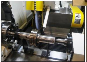
Weldon designed crossaxis pneumatic rotary dressing system generates a full radius on conventional abrasives. Renishaw probe is used to establish lateral position with part mounted on a custom between centers arbor. The probe is also used to measure the OD for automatic depth control.
