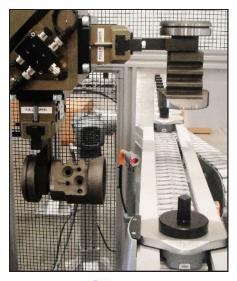
Weldon's automation package incorporates a heavy-duty 2-axis gantry load/unload system, dual gripper tooling with a pneumatic coupling for crash protection, and a powered loop conveyor with puck system for part presentation and exit. The machines can run either worms or racks with minimal change-over. Size is controlled by (2) table mounted gage heads that can be applied post-grind and provide feedback to the machine's control for size compensation as required.
