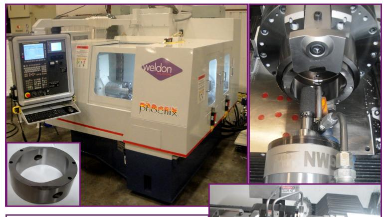
Hydraulic pump manufacturer calls on Weldon for a second **Phoenix** ID cam grinder. This new machine features X and Z axis linear motors and a FANUC control with high-speed cycle cutting. The result was a system that could produce higher quality cams with up to a 50% improvement in productivity. Work holding was accomplished with a custom face clamping chuck.
