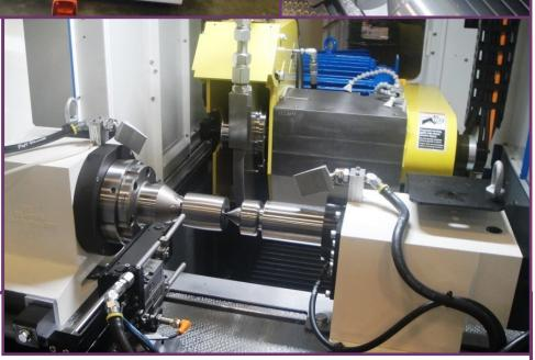
**Dittel** acoustic sensor, **SBS** automatic wheel balancer, **Neidlein** face driver, **Marposs** in-process gage, **Barnes** coolant system, **Turmoil** coolant chiller, **Absolent** mist collector, **FANUC** 32*i* BT CNC control.
