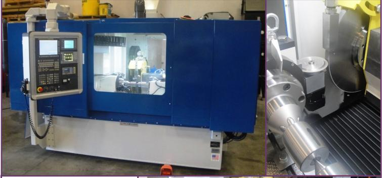
A rotary bearing manufacturer called on Weldon to build a roller OD grinder for a large bearing family. The machine features an X-axis linear motor for smooth transitions when grinding the crowned OD with a convex grinding wheel face in a single pass profile interpolation cycle. This allows grinding of all part numbers with the same tooling.
