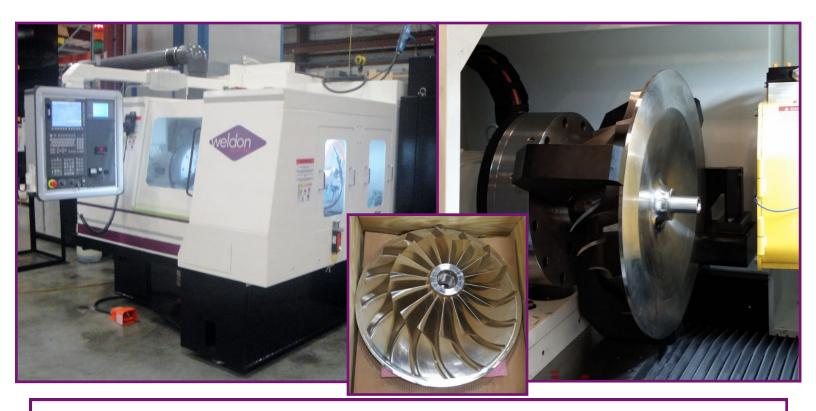
Weldon's **Phoenix** is selected to replace a Jig Grinder for OD and ID polygon grinding. This machine features a custom 18" pneumatic chuck for Impeller OD & Pinion ID work support. Jig grinder accuracy and high productivity rates were made possible through the use of X and Z axis linear motor technology. Enclosure modifications helped address the need for 25.5" swing capacity.
