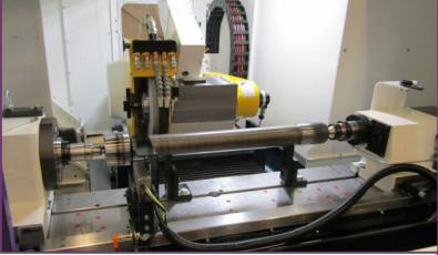
lects **Weldon Solutions** for grinding multiple diameters on various axle shafts. This is the first re-designed **midas** CNC grinder to be installed. The new machine features a Z-axis linear motor, increased Z-axis stroke, shear-damper base updates, dual front enclosure door system, and a new 5" stroke hydraulic tailstock with smart cylinder positioning and gear reducer for easy taper compensation. In this process, bearing journals on both
