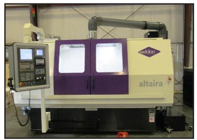
The US division of a major compressor company selected the Weldon Altaira for grinding shaft diameters and shoulders on both ends of a rotor in a single cycle. This was accomplished using a straight approach vitrified CBN grinding wheel, relieved on both sides.
