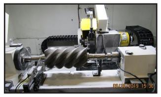
The Weldon Altaira has a compound slide design allowing it to grind parts up to 40" (1m) long while maintaining a small footprint. The Z-axis features a FANUC linear motor and the X-axis can be a linear motor or ballscrew drive depending on the application.
