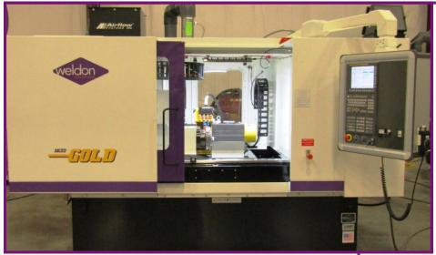
An Ohio based producer of rod steel has accepted delivery of a new Weldon model 1632 GOLD OD CNC grinder. In this application, a carbide mill roll is supported by a heavy duty slip-fit arbor assembly. A full radius,
