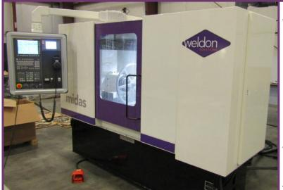
A Midwest based manufacturer of industrial meat processing equipment has accepted delivery of a new Weldon model Midas 120A OD CNC grinder. In this application, an angled grinding wheel is form dressed with a stationary diamond tool
