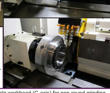
This machine is equipped with a programmable workhead (C-axis) for non-round grinding. The workhead also features a swivel base with rotary position sensor for digital readout of swivel angle. Additional features include Helical Interpolation, Z-Axis Chopping, Modulating Wheel Speed for chatter control, Weldon's EZPunch software, and MT Connect compatibility.
