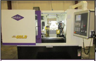
A western PA based mold and die maker selects Weldon for their Carbide OD, ID, and non-round grinding application. The model 1632 GOLD will swing and grind parts up to 16" in diameter and has the power and stiffness needed for the special demands of Carbide grinding.
