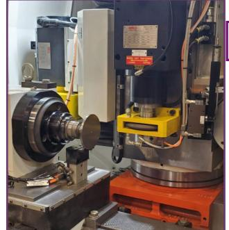
In place of a primary flat, for the 3rd operation, a notch can be ground with the fixed, vertical sub-spindle using a pre-formed wheel.
