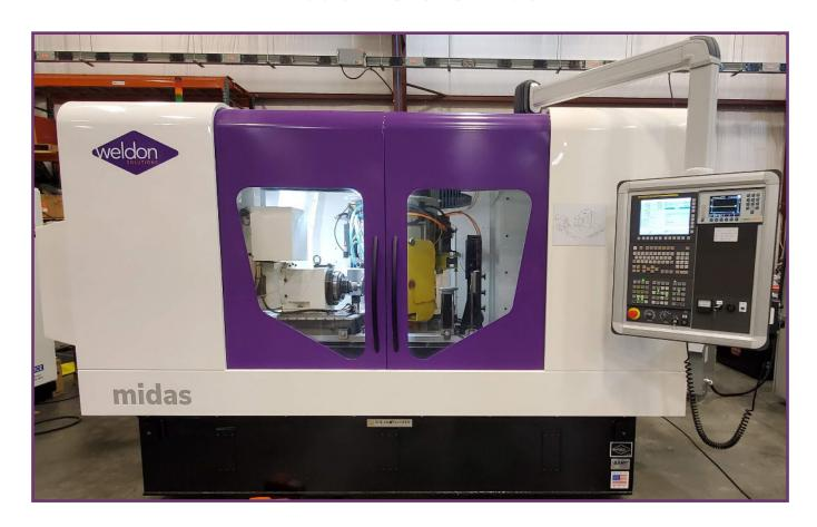
A leader in Silicon Carbide (SiC) Wafer technology has once again come to Weldon for solutions to their unique SiC boule (ingot) grinding requirements. In this application, Weldon's multi-spindle, turret based wheelhead design on the Midas platform allows for OD, Face, Flat, Notching, and Angled-Plane End Face grinding all in the same cycle.
