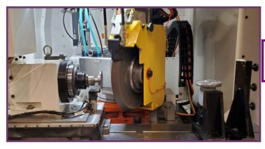
In the 1st operation, the main spindle angular approach grinding wheel is used to grind the OD and then the flat end face (dome).
