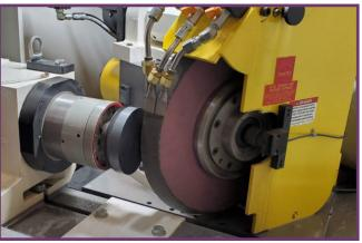
Silicon wafer production cost is greatly reduced with Weldon's unique multi-spindle design allowing OD, Flat, and Face grinding in the same operation. Other processes that can be incorporate into a common platform include formed notch and angled-plane end face grinding.
