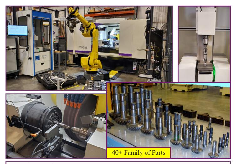
A manufacturer of power transmission components has added their 4th **Weldon model Midas 324A** machine to their grinding department. This fully automated workcell also features a **Jenoptik** optical gage for post-process inspection, providing feedback to a **Movomatic** in-process gage for automatic control of size tolerances under 10 microns.
