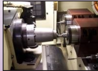
5C collet chuck with drawbar and pneumatic actuator
