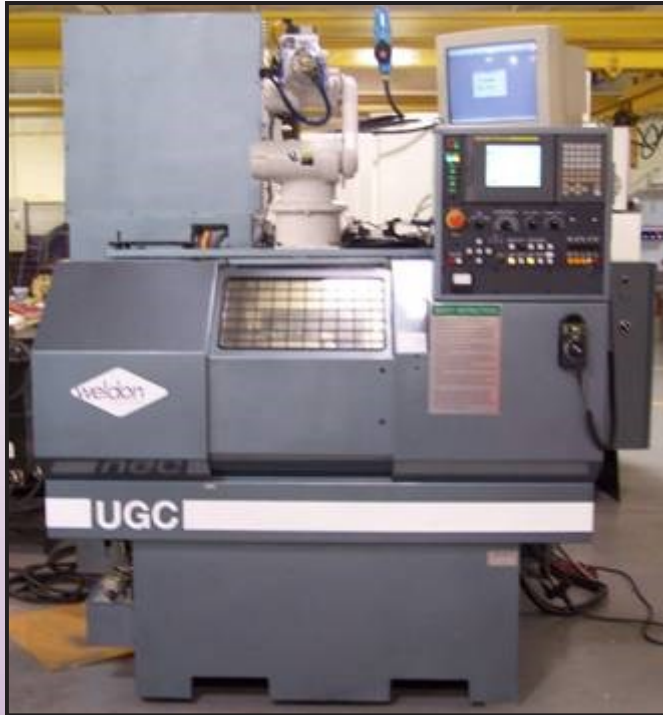
Multi-purpose grinder for OD, Face, and ID grinding in a single set-up
