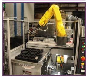
This Weldon model AGN4 incorporates a full turnkey for over 40 different part numbers. Machine tending automation features a 6-axis robot & a dual pallet tray system for part presentation and exit.
