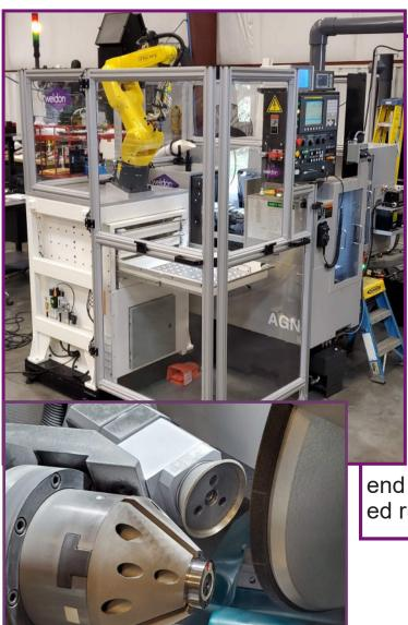
A global manufacturer of heavyduty construction equipment has selected Weldon to be the supplier for their fuel injector solenoid valve face grinding needs.
