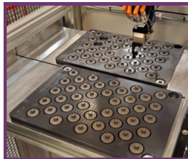
Dual Pallet Station w/ Vertical Presentation
