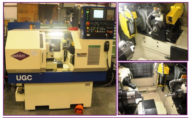
A major mid-west X-ray equipment manufacturer selects the Weldon model **UGC** in a dual spindle configuration, with a single ID and OD spindle, for grinding a wide variety of parts made from proprietary exotic materials.
