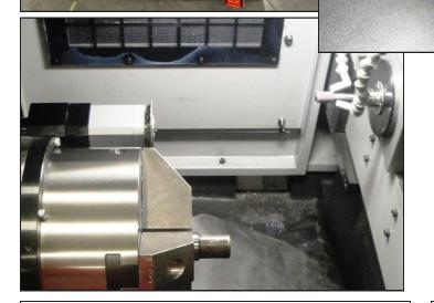
Electric rotary dresser for automatic dressing of both conventional and super-abrasive grinding wheels.
