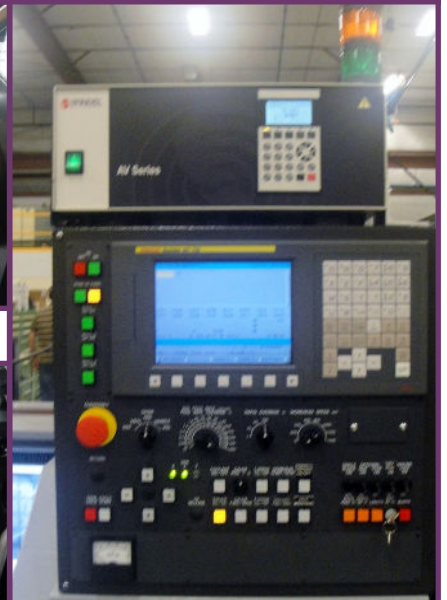
FANUC 0i TD CNC control and dresser drive panel
