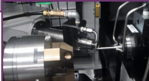
Pneumatic positioning slide for dresser
