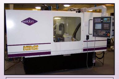
High production aerospace grade bolt grinding with a single vitrified CBN wheel configuration for all part sizes.
