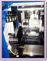
OD spindle in straight wheelhead configuration for round and non-round grinding using both conventional and CBN abrasives
