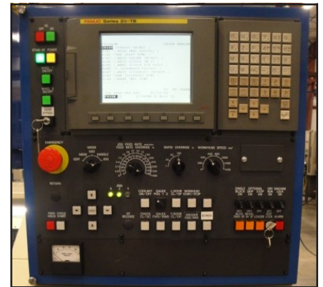
Operator control panel featuring a FANUC 21i CNC control
