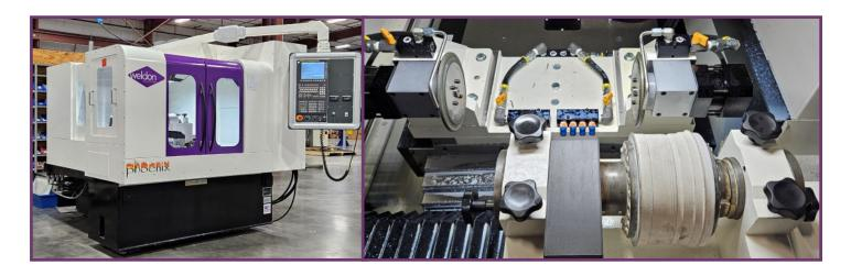
An aerospace component manufacturer was looking to replace an aging offline grinding wheel dresser. The grinding wheels are used in their manufacturing processes on a large number of existing grinders. Their current system is 20+ years old and is not very efficient at rough and finish dressing their aluminum oxide grinding wheels and is no longer able to be built by the original manufacturer.
