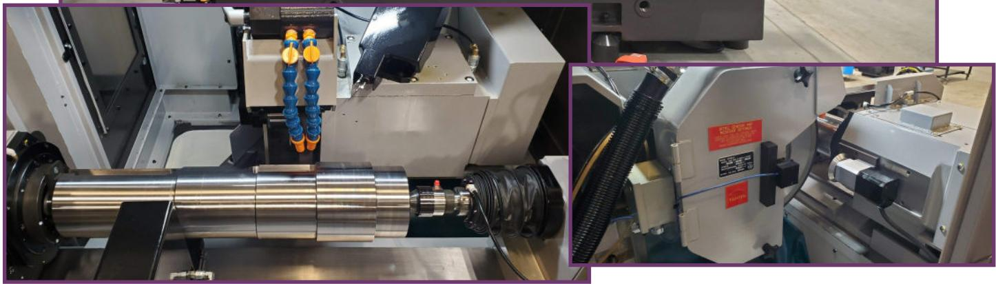
A leader in the Power Transmission industry has selected Weldon's **G300** grinder to process shafts for their gearbox and speed reducer products. This model is capable of up to 1000mm between centers necessary to be able to grind the vast range of length parts (100-1000mm). Configured with a fixed straight approach wheelhead, this machine uses vitrified CBN superabrasives for plunge grinding diameters, under in-process gage control, and side wheeling faces.
