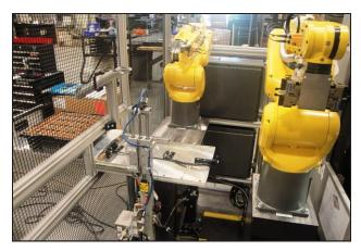
Weldon designed dual robotic automation turnkey with (1) robot tending the pre-gage station that measures the armature counterbore depth. The 2nd robot tends the grinder that grinds the pin end face to precisely match the output from the armature gage to a 5 micron total tolerance. Part presentation and exit via pallet tray designed to keep parts in matched pairs.
