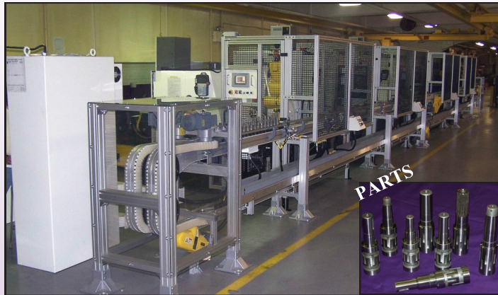
Master Cell Controller with Allen Bradley PLC
