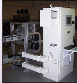
Master Cell Controller with Allen Bradley PLC
